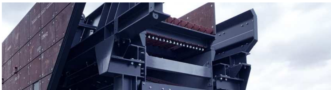
BE1430 drive – vibrator shaft, counterweights and bearing housings.
